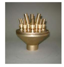
Distribution boxes are made of cast and machined brass. They are specially designed to put cover on different nozzles that (depending on type and situation) will create various ornamental water effects. Cover could be produced undrilled and unthreaded or completely drilled and threaded by customer requirements.
